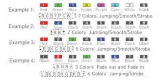
Notes: If not using all eight colors in a scene, the remaining color spaces must be set with the light off.
